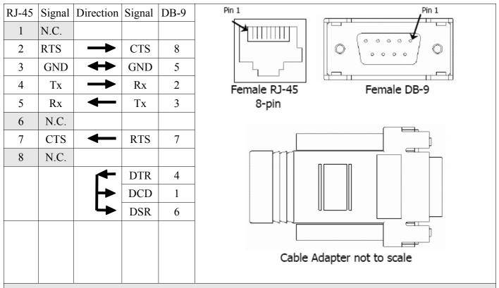
These pins are not connected on the RJ-45 Connector. They are reserved for DTR, DSR and DCD functions!
